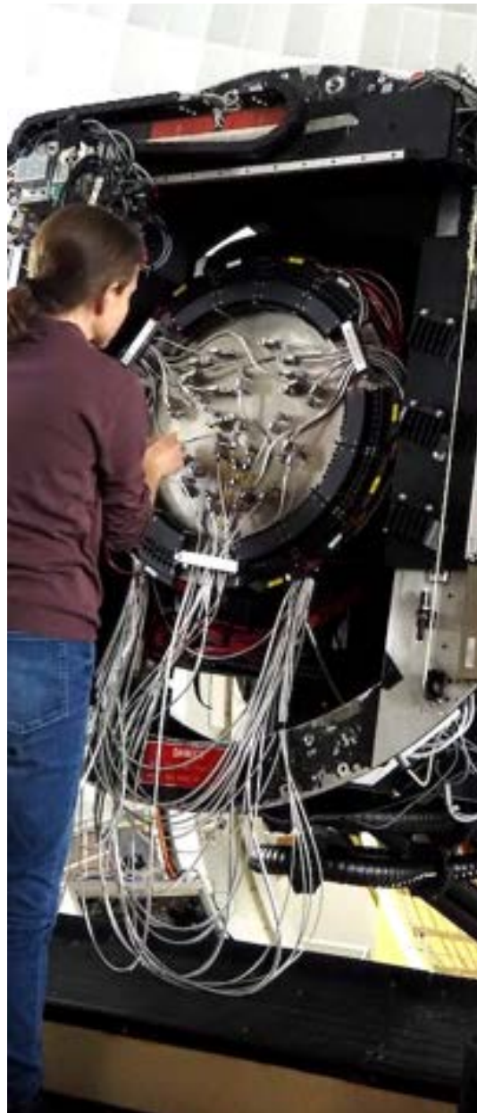
The field plate of the Hector instrument mounted on the Anglo-Australian Telescope showing the precisely positioned magnets holding the end of each hexabundle (group of optical fibres).| Credit: Jesse van de Sande & the Hector Team
